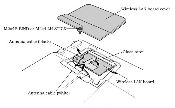
Figure 4-10 Removing the wireless LAN board
